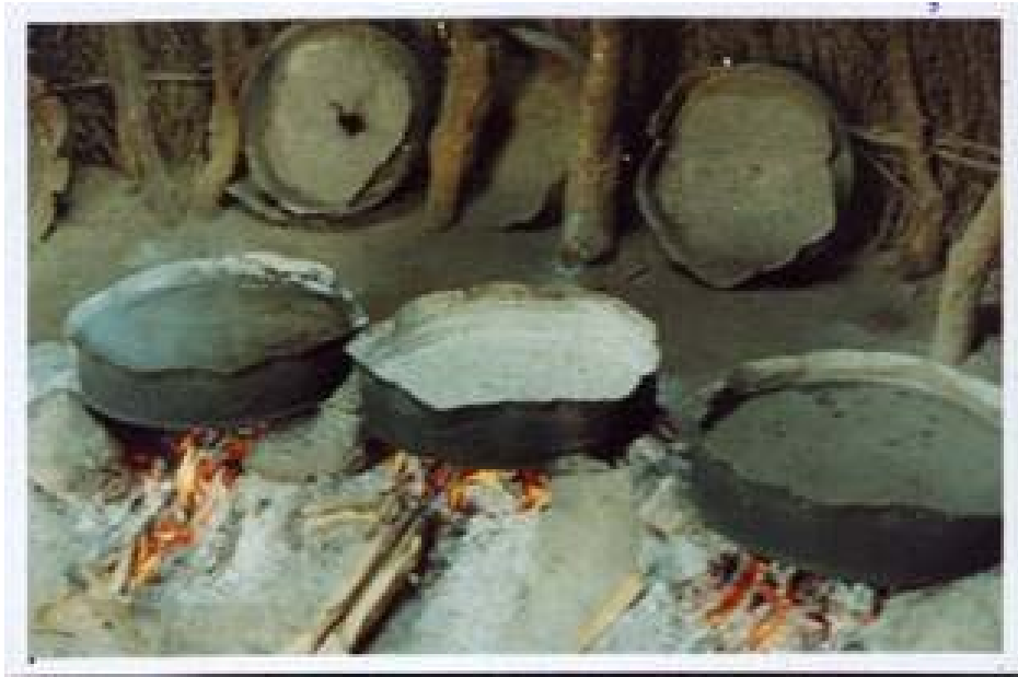
Photo 6.1: Boiling brine in the traditional salt extraction process in El Ga'a
